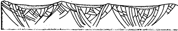
FIGURE 18-43 Diagrammatic cross section showing the possible pattern of the block faulting in the Basin and Range Province that might have been responsible for lateral extension of the crust.
