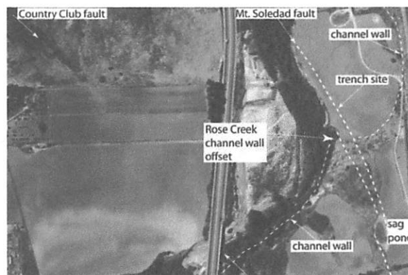
Figure 5. 1928 aerial photograph (Fairchild collection) showing the location of the Lindvall and Rockwell (1995) trench site on the Mt. Soledad strand. Note the vegetation lineament across the Holocene terrace to Rose Creek, suggesting that the Country Club fault may be active in this area. The Rose Canyon fault ( sensu stricto ) is off the photograph to the northeast.
