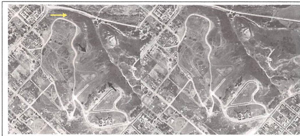
Figure 4. San Diego County 1928 photographs of Presidio Park area. Black arrows point to northeast trending fault scarps bounding the Presidio Park Graben. Yellow arrow points to possible right-lateral offset of valley wall. Geologic map Figure 1 shows an uphill-facing possible fault scarp and closed drainage south of the road below the yellow arrow that may be evidence of a landslide or an active fault.
