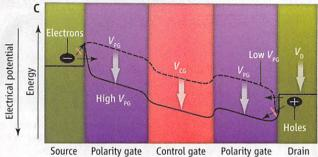
Meanwhile a relatively high complementary barrier is needed to suppress leakage current from the "reverse" tunneling by carriers of opposite signs at the drain in the OFF state.
