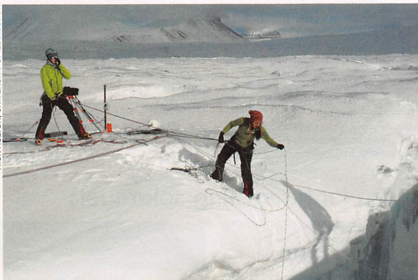
To study glacier dynamics , postdoc Faezeh Nick (right), secured by PhD student Heidi Sevestre, lowers pressure and temperature sensors into a crevasse in Kronebreen, a glacier about 100 km northwest of Longyearbyen.
