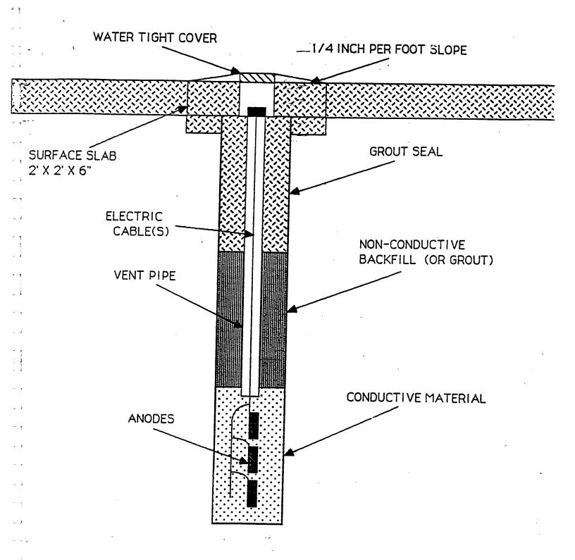
CATHODIC PROTECTION WELL CROSS SECTION
