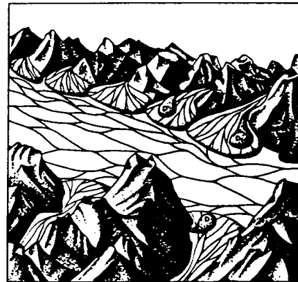
Figure 2 Block diagram of alluvial fans tributary to a braided river in a trunk valley. D) debris flows.
