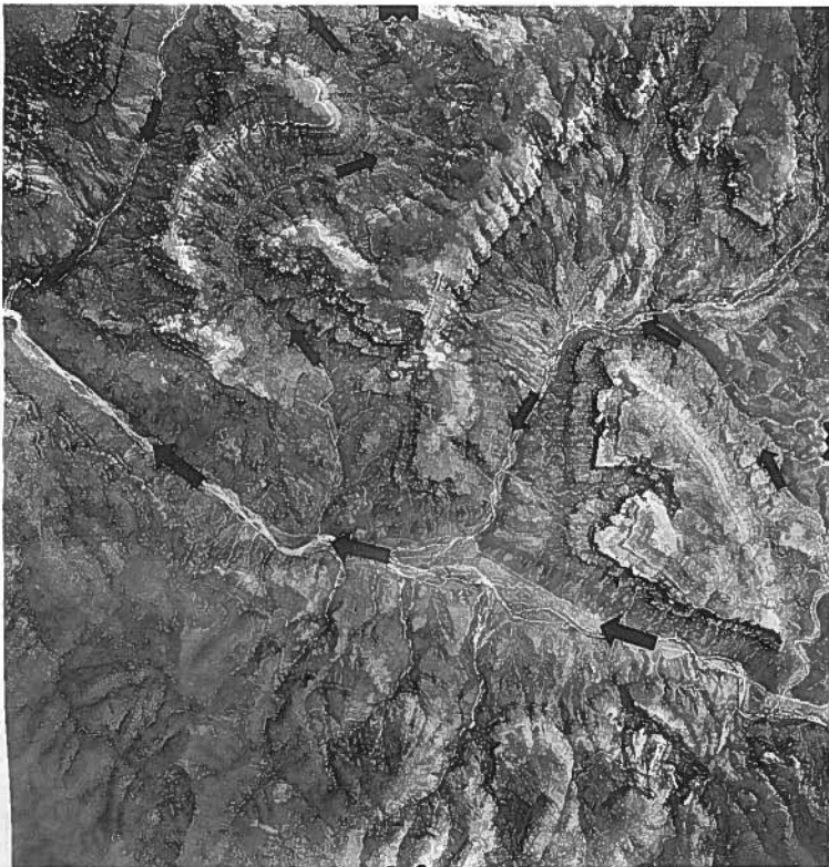
FIGURE 14.13. Deeply incised Laramide paleovalleys in the Peach Springs Canyon area, western Grand Canyon, Arizona. The two meander loops ( small arrows ) are older and less deeply incised than the Peach Springs paleocanyon ( large arrows ), which is colinear with the Hurricane fault. Offset Early Tertiary rocks along the floor of Peach Springs Canyon reveal that Late Cenozoic normal faulting postdated incision of both channels. Arrows show paleocurrent directions. (U.S. Geological Survey photograph.)
