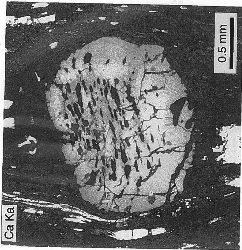
FIGURE 2.8. Electron microprobe, Ca Ka map showing compositional zoning in a single garnet crystal from mile 82. The thin-section view is approximately vertical and perpendicular to NE-striking S2 foliation. Note that the core of the garnet overgrew a slightly folded (S1) fabric. This early fabric was folded and transposed into the vertical S2 orientation now seen in the garnet rim and outside of the crystal. The increasing Ca content of the garnet, along with the composition of other associated minerals, suggests that the garnet core grew as temperature and pressure increased. Peak conditions of approximately 550°C and 6 kbar (20-km depths) were reached during the growth of the outer part of the garnet, but the compositions of the extreme garnet rims indicate that pressures decreased during the final increments of growth. The composition of matrix minerals indicate that the final matrix recrystallization occurred at conditions near 550°C and 3 kbar (10-km depths). Thus, this one garnet crystal and its matrix record increasing pressures and the subsequent decompression from 20- to 10-km depths all during D2 deformation. The compositional map was collected on a Cameca SX-50 electron microprobe at the University of Massachusetts.
