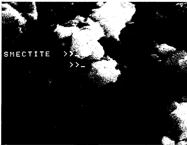
Figure 9 —SEM photomicrographs of clay minerals (identified by energy dispersive x-ray analysis) in Austin Chalk. (a) Arrows indicate large, amorphous clay mineral aggregate in finer grained chalk matrix. Dessau chalk (DRT) porosity plug; bar scale = 10 \mu\text{m} . (b) Small smectite clay fragments on shear fracture surface of experimentally deformed sample DRT-2; bar scale = 1 \mu\text{m} .
